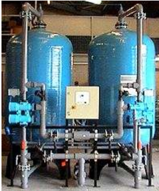
Ion exchange plant
